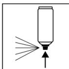
After painting, turn the can upside down and spray for 3 - 5 seconds to clean the valve.
