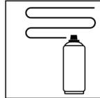
Apply several 1 - 2 light spray passes to the edge of the blending area immediately after application of the 2K clear coat or 2K topcoat to achieve a smooth transition.
